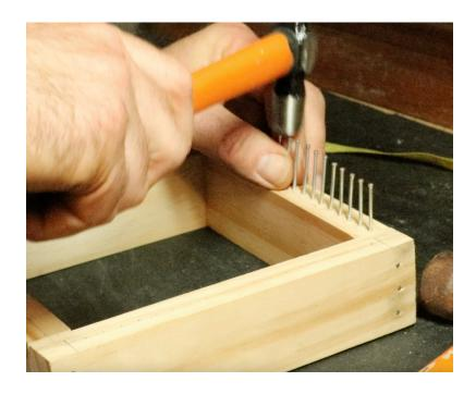
Take your time with this step. Your nails do not need to be perfectly straight, just try to be consistent with the spacing and angle.
