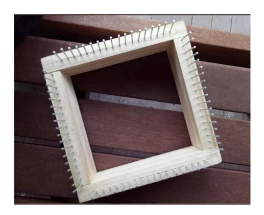
These pieces were secured together with 3 nails at each end you could also use wood glue to secure the frame before hammering in the nails.
